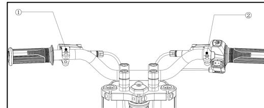
For model E500: Use a tool to remove the brake lever fastening screws. Install the brake lever as shown in the diagram and pre-tighten. Move the left brake lever to 20-25 mm from the handlebar grip and adjust to a suitable angle. Use a tool to tighten screw ①(8-10 N.m). Move the right brake lever to 10-15 mm from the throttle grip and adjust to a suitable angle. Use a tool to tighten screw ②(8-10 N.m).
