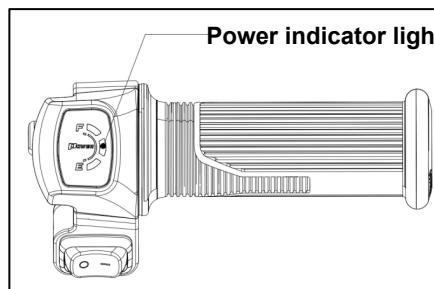
The diagram shows the battery display function. The meter has three lights; when all three are lit, the battery is over 75% charged. When only one light remains and it changes from green to red, it indicates that the vehicle needs to be charged to continue riding.
