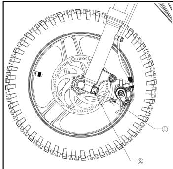
Remove the disc brake mounting screw from position ①. Rotate the disc brake to position ② and align the center hole. The disc brake caliper should align with the disc on the front wheel. Use the mounting screws to tighten the disc brake(8-10 N.m).
