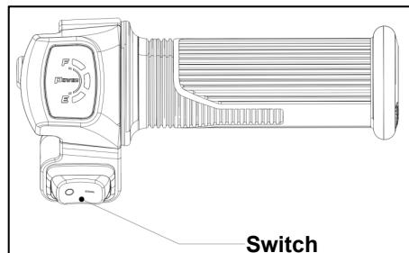
The diagram shows the vehicle's power button. To operate the vehicle, use this button to turn the power on or off. The "I" position indicates that the vehicle is on, and the "O" position indicates that it is off. When the display lights up, the vehicle is in the on state; when the display lights go off, the vehicle is in the off state.
