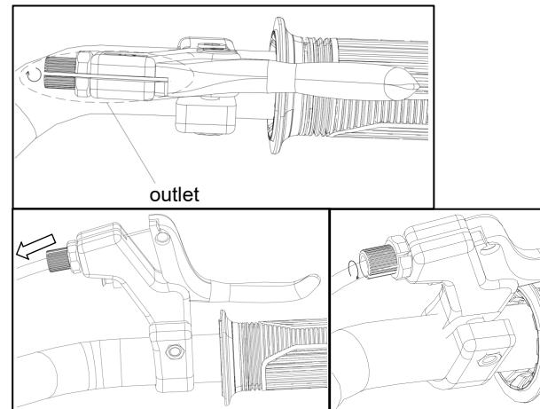
For models E150,E250,E350: Rotate the brake lever adjustment screw to align the opening with the cable outlet. Insert the brake cable head into the cable head seat of the brake lever. Pull the cable core into the brake lever outlet with a force of 10-15 kgf. Finally, rotate the opening nut half a turn to misalign.
