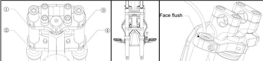
Use a tool to loosen the four fastening screws as shown in the diagram.Press the front shock absorber down until it is flush with the upper connecting board.Tighten the four screws(11-13 N.m).
