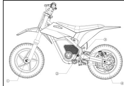
Before using this vehicle, you should inspect all fasteners as shown in the diagrams to ensure they are not loose. This is essential to prevent any safety hazards due to loosened fasteners.
