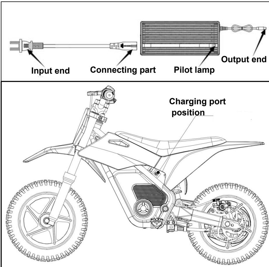
To charge this product, connect the charger to the input end, then plug the input end into a household socket, and insert the output end into the charging port shown in the diagram to start charging the vehicle.
