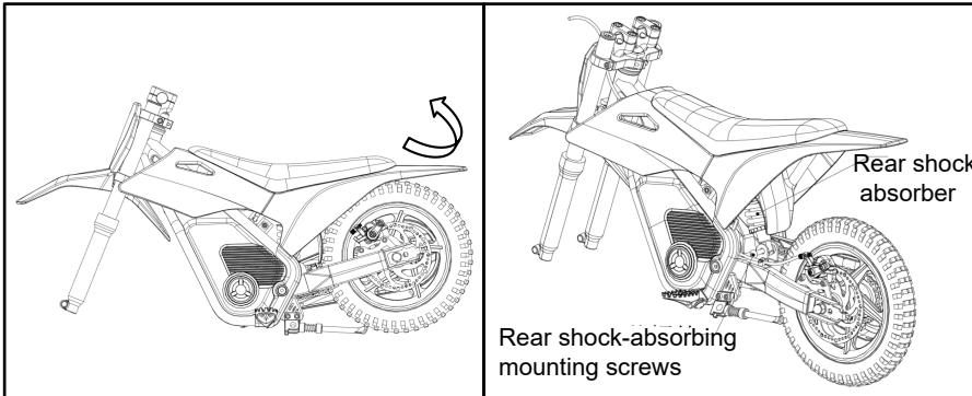
Lift the rear of the bike.Align the lower end of the rear shock absorber with the mounting hole on the rear fork of the frame.Use a tool to tighten the rear shock absorber mounting bolt(10-12 N.m).
