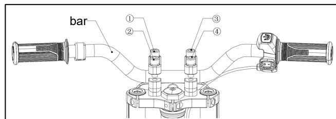
Use a tool to remove the four screws from the handlebar stem. Install the handlebar as shown in the diagram. Adjust the handlebar angle to a comfortable position. Use a tool to tighten the four screws on the handlebar stem(10-12 N.m), ensuring the gap between the handlebar stem and the lower stem is even.
