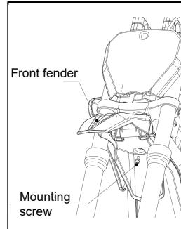
Align the front mudguard limiter buckle towards the back and attach it to the lower fork board.Insert the limiter post of the front mudguard into the inner limiter hole of the number plate.Use a tool to tighten the front mudguard screw into the lower fork board mounting hole(8-10 N.m).
